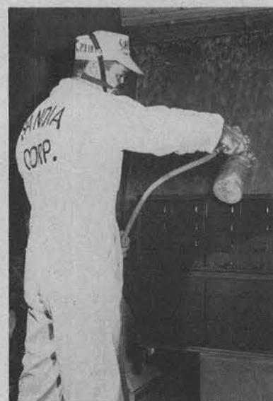
**WATERFALL AND SPRAY** go together in an unusual way in the painting section. A face mask makes sure this man doesn't breathe in any of the mist-like paint spray and at the same time water pouring down the wall in the background, plus a suction fan, removes the paint from the air.
